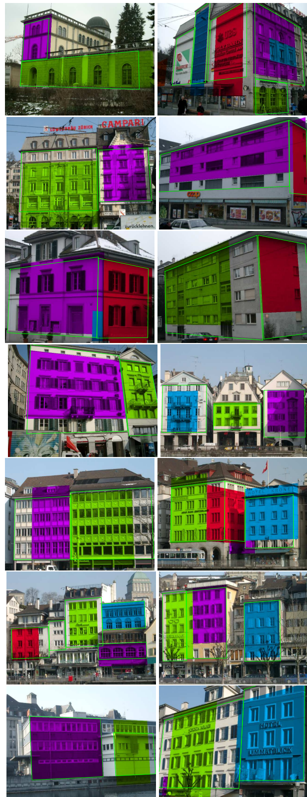
Figure 10: Example results of the whole facade recognition method obtained on the Zubud database. The green polygons are the ground truth facades. All the facades shown in this figure were correctly recognized.
