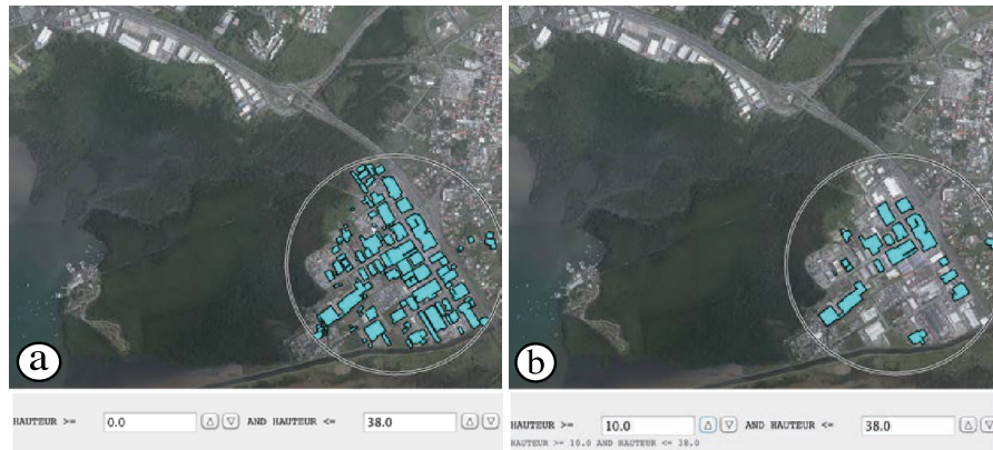
Figure 4. (a) Highlighting all buildings in a given geographical area using color compositing. (b) Dynamically adjusting query parameters to highlight buildings taller than 10m only.
