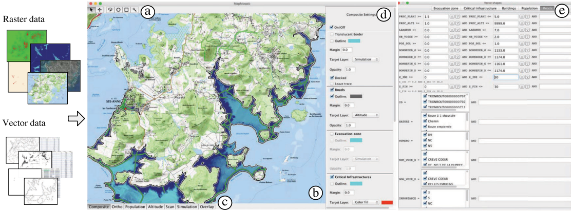
Figure 1. A proof-of-concept implementation of the MapMosaic dynamic compositing model and interaction techniques. (a) Toolbar to navigate the map, and to create & select areas. (b) Map viewer. (c) Access to individual layers. (d) Compositing area inspector. (e) Query builder for compositing region filters.
