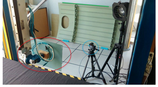
Fig. 5. Experimental setup: the mirror (red circle) is mounted on the robot end effector; the camera (blue circles) observes the target (green line) as its reflection in the mirror.
