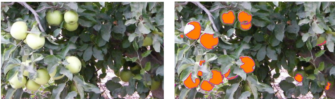
Fig. 11. (Left) Typical image. (Right) Detected "seed areas" (in orange)
