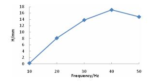
Fig. 6. Seeds accumulation heights under different frequencies
