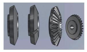
Fig. 2. Creating process of the bevel gear
