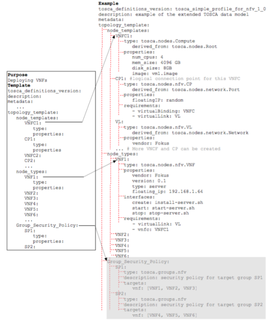
Fig. 4. The extended TOSCA data model with security policy specification (highlighted in grey)
