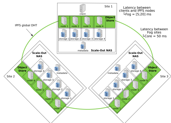
Fig. 1: Topology used to deploy an object store on top of a Scale-Out NAS local to each site.
