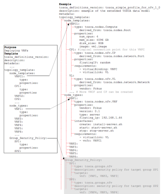
Fig. 4. The extended TOSCA data model with security policy specification (highlighted in grey)
