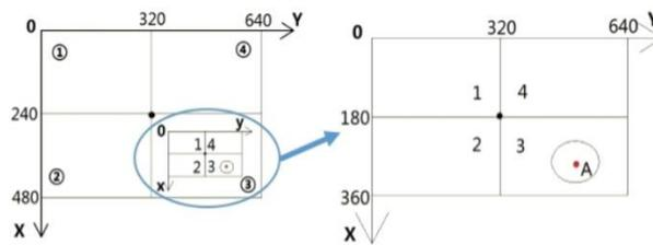
(a) Microsoft camera image coordinate system (b) Kinect sensor image coordinate system
