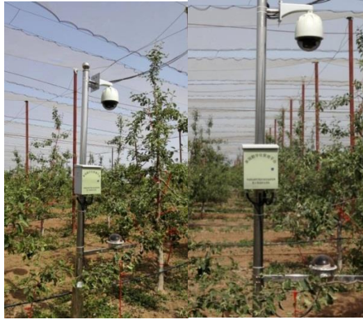
Fig. 2 Physical picture of the surveillance pole
