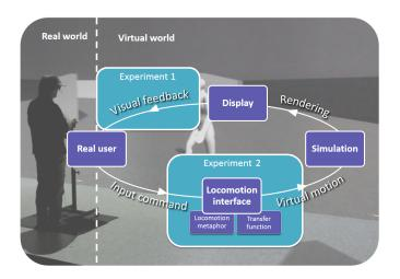
Fig. 2. Illustration of the interaction loop between a real user and a virtual character in an immersive environment
