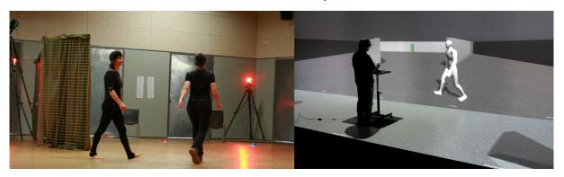
Fig. 1. The objective of this article is to evaluate whether small scale interactions during locomotion between a real user and a virtual human (right) are similar in virtual conditions in comparison with real ones (left).
