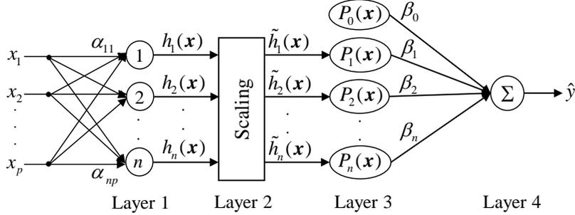
**Fig. 3** The Legendre polynomial feedforward neural network.
