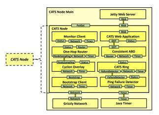
Fig. 11. The architecture of the CATS Node. We omit the channels for clarity. In this scope, all provided ports are connected to all required ports of the same type.
