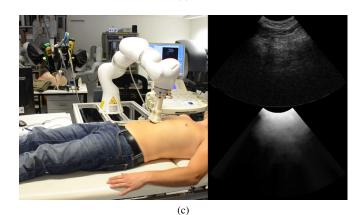
Fig. 14. Confidence-optimized tele-echography on a human volunteer – frontal abdominal scan – normal breathing. (a) Initial position. (b) The operator moves the probe towards the right side of the patient (t = 21 s). (c) The operator moves the probe back to the center of the torso (t = 51 s).
