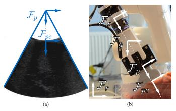
Fig. 2. Coordinate frames attached to the ultrasound probe, represented (a) on the ultrasound image and (b) on a picture of the robotic system.
