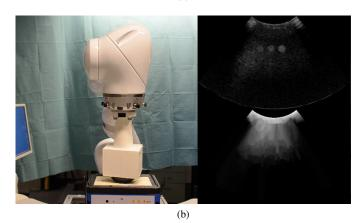
Fig. 5. 3D global confidence-driven control. (a) Initial configuration – the probe is not fully in contact with the phantom. (b) The system has converged, and the image quality is higher.
