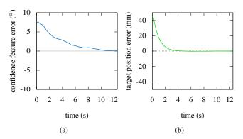
Fig. 8. Convergence of the target-specific confidence-driven control in a static environment. (a) Confidence feature error  $\theta_c$  in degrees. (b) Target centering error  $e_t$  in millimeters.
