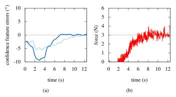
Fig. 6. Convergence of the global confidence-driven control in a static environment. (a) Confidence feature errors  $e_{\theta}$  (—) and  $e_{\phi}$  (—) in degrees. (b) Contact force  $s_f$  in Newtons.
