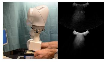
Fig. 9. 3D global confidence-driven control -A shadow is generated using a paper band, which is inserted between the probe and the phantom by the experimenter. The system reacts automatically by reorienting the probe.
