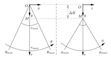
Fig. 1. Imaging geometry of a three-dimensional convex ultrasound probe. (left) Front view, also corresponding to the imaging geometry of a 2D probe. (right) Side view, showing the range of the motor.
