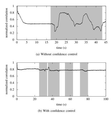
Fig. 13. Evolution of the normalized correlation between the tracked target and the initial template, (a) without and (b) with confidence control.
