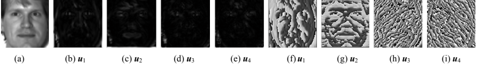
Fig. 2. (a) Original face image. (b)-(i) magnitudes and phases of STFT at frequencies u_1, u_2, u_3 and u_4 from left to right.
