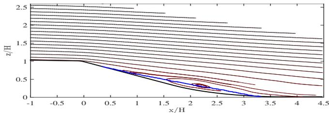
Fig. 2. Streamlines for the flow under continuous actuation
