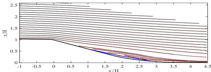
Fig. 3. Streamlines for the natural flow without control. The blue line represents the border between the reversed flow (negative streamwise velocity, region of the flow below the line) and the freestream (positive streamwise velocity, region of the flow above the line). In the controlled case Fig. 3 the recirculation region is shown to be drastically reduced and the flow almost fully reattached to the wall.
