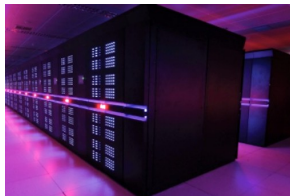
Tianhe-2, China, #2 34 Pflops Fat tree 32,000 × 12 cores + 48,000 Xeon Phi
