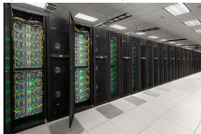
Stampede, United States, #20 5 Pflops Fat tree 6,400 × (8 cores + 1 Xeon Phi)
