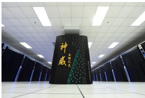
Sunway TaihuLight, China, #1 93 Pflops Custom five level hierarchy 40,950 × 260 cores
