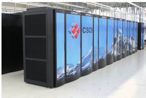
Piz Daint, Switzerland, #3 20 Pflops Dragonfly 5,272 × (8 cores + 1 GPU)
