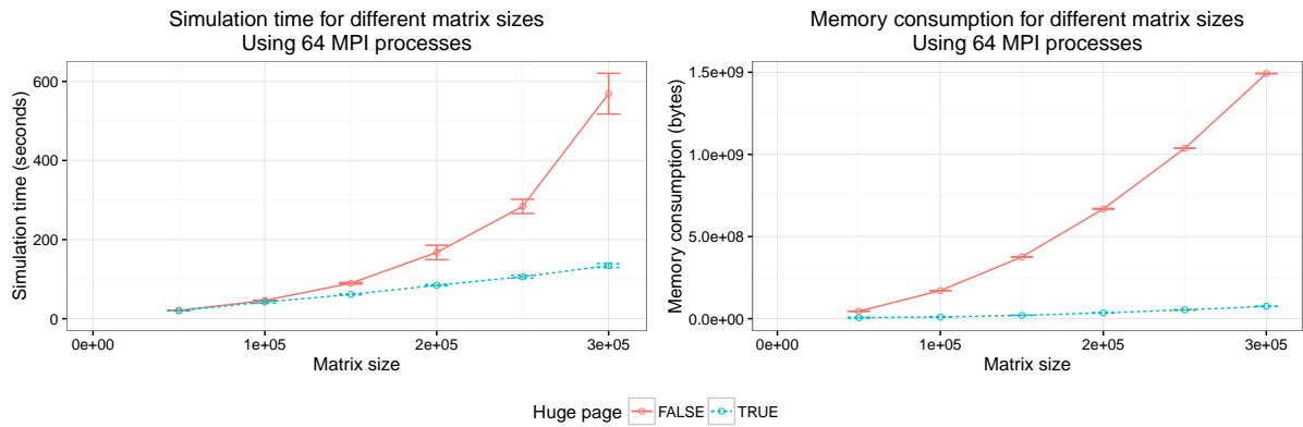
Figure 4.9 – Effect of huge pages on the simulation time and the memory consumption
