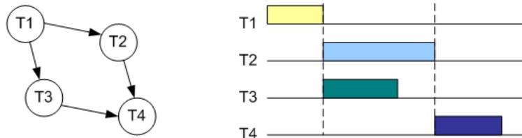
**Fig. 1.** Applications described as a directed graph and the associated task activation diagram
