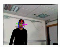
green arrow: person's self-motion magenta arrow: motion due to robot-motion
