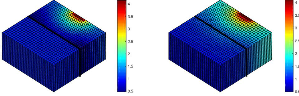
Figure 4: Test case 1: Robin interface conditions, capillary pressure  $\pi(u(t), \cdot)$  for  $t = 6.6$  and  $t = 15$
