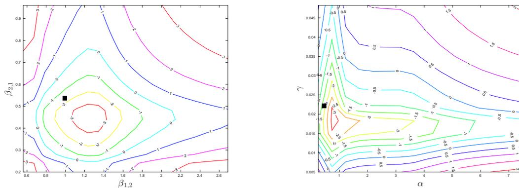
Figure 10: Test case 1: Domain decomposition error estimator  $\eta_{\text{dd}}^{k,m}$  as a function of the free parameters after 4 iterations of the OSWR of the two-sided Robin-OSWR method (left) and 3 iterations of the optimized Ventcell-OSWR method (right)
