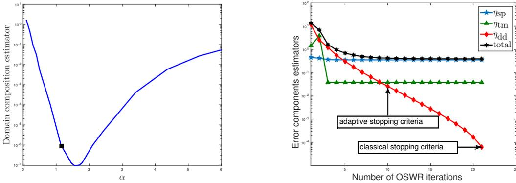
Figure 5: Test case 1: Domain decomposition estimator  $\eta_{\text{dd}}^{k,m}$  after 25 Robin-OSWR iterations as a function of the parameter  $\alpha$  (left) and evolution of the spatial, temporal, and domain decomposition estimators as a function of the number of Robin-OSWR iterations until  $\text{err}_{\text{OSWR}}^{21} \leq 10^{-6}$  (right)
