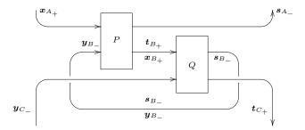
The loop is executed using the trace operation defined in the preceding section. The syntactic view of this operation is:
