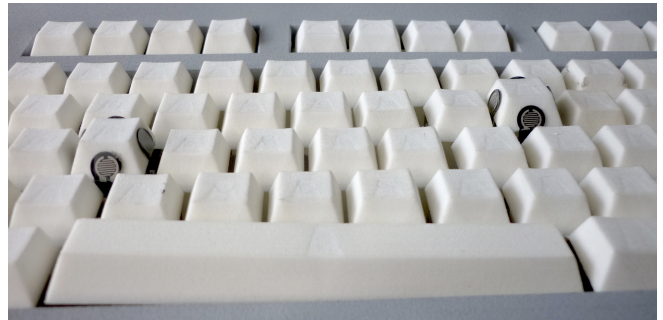
Figure 1: Métamorphe is a keyboard with actuated keys, which can either be up or down.
