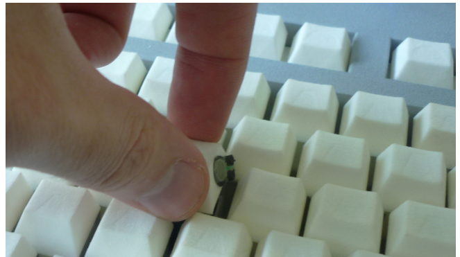
Figure 2: Raised keys have new affordances. They can be pushed or pinched.
