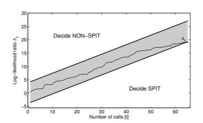
Fig. 1. An example run of SPRT. The log-likelihood ratio  $A_t$  starts at t = 1 in the region between the decision boundaries and, with each new sample observed from the unknown source, performs a random walk over time. Eventually it will cross over one of the decision boundaries and either enter the region marked "decide SPIT" or enter the region marked "decide NON-SPIT".
