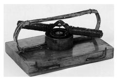
Figure 2.2: The first electro-motor
