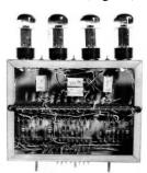
Figure 6.8: The logic unit of EDVAC
