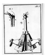
Figure 1.6: The first model of Kempelen's speaking machine, right and left lungs (A,B), windpipe (CD), larynx (H), tongue (L), pharynx (R)
