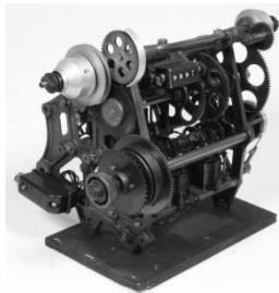
Figure 4: Electro-mechanical Totalisator: ‘Julius Horse Adder’, c 1926
