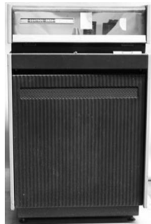
Figure 9: Disk drive; part of a Control Data model 3200 computer system Photo courtesy of Museum Victoria
