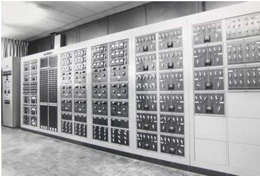
Figure 6: Network Analyser – Westinghouse Electric Corporation Photo courtesy of Museum Victoria
