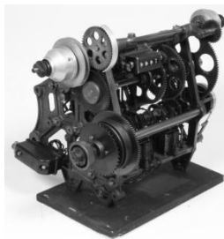
Figure 4: Electro-mechanical Totalisator: ‘Julius Horse Adder’, c 1926
