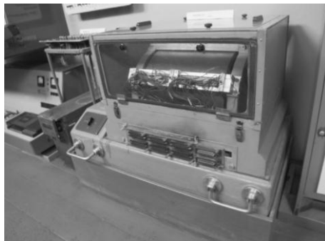
Magnetic DRUM – 'hard disk'
