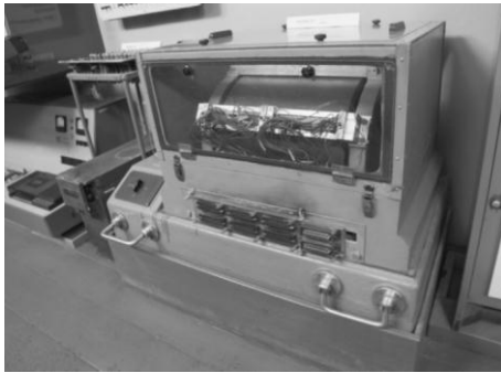
Magnetic DRUM – ‘hard disk’
