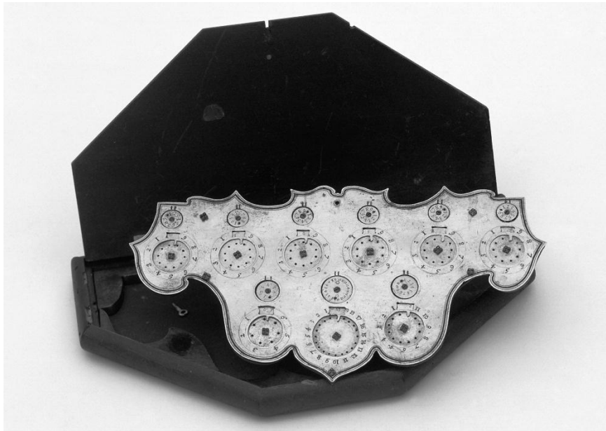
Fig. 3 - Dial adder attributed to Tito Livio Burattini (Museo Galileo, Florence, - Photography Franca Principe)
