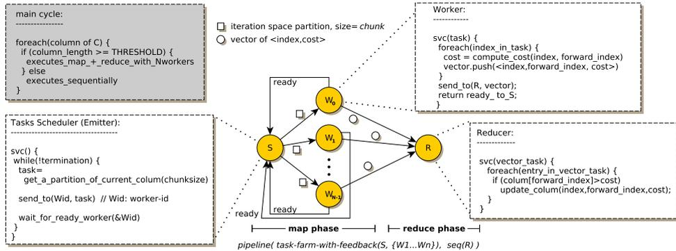
**Fig. 2.** The FastFlow skeleton used in PWHATSHAP. Each entity is a concurrent thread. The Emitter ( $S$ ) produces and schedules tasks towards a pool of Workers ( $W$ s). Each Worker sends results to the Reducer ( $R$ ) and asks for new tasks from  $S$ .
