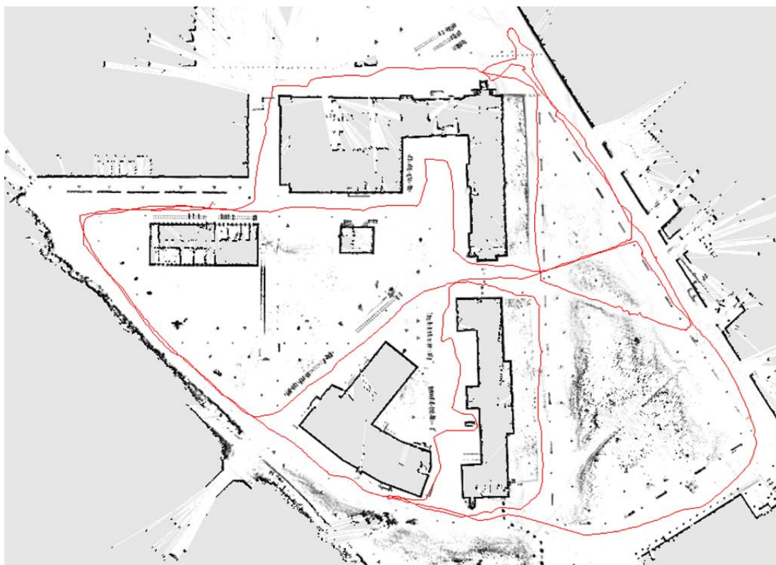
Figure 2.10: Example of a map of the Freiburg University campus constructed with the SLAM-algorithm proposed in [17]. According to the authors, the robot traverses an area of approx. 250m x 250m on a trajectory of a length of 1.75km. 30 particles were used. Figure taken from [17].
