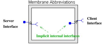
Figure 3: Abbreviations for matching external/internal interfaces
