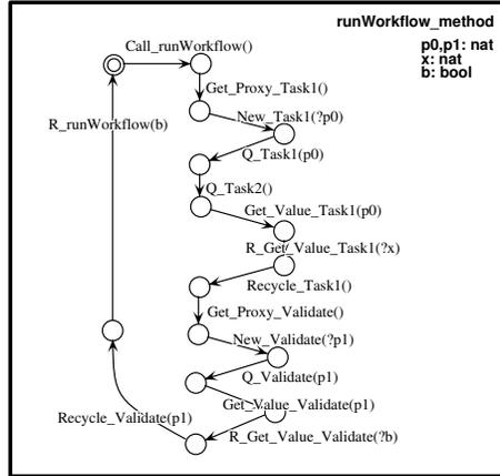
Figure 14: pLTS model for the runWorkflow method
