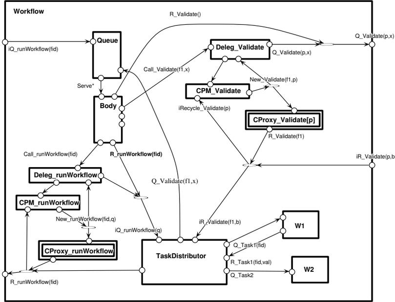
Figure 15: pNet model for the Workflow composite component
