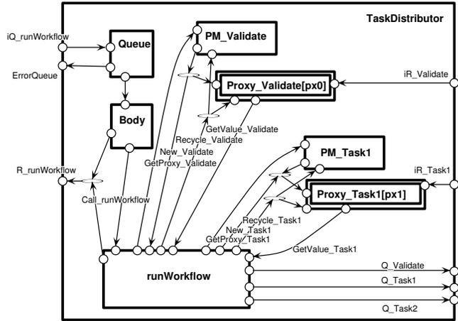
Figure 13: pNet model for the TaskDistributor Primitive component
