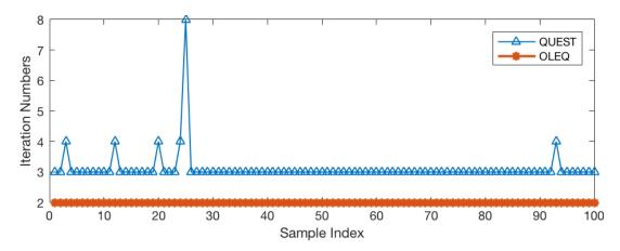
Figure 1: Iteration numbers of QUEST and OLEQ in face of an extreme case.
