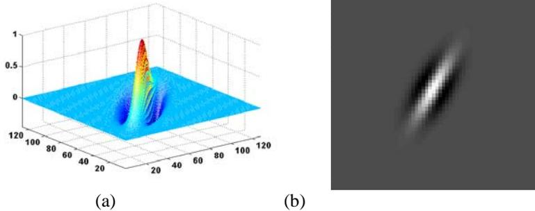
**Fig. 1.** (a) Appearance of anisotropic filter(2D);(b) Sample anisotropic filter with a rotation of  $2\pi/3$  radians and scales of 3 and 9
