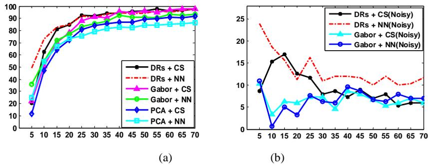
**Fig. 7.** Performance Original palmprint database under noise corruption (a) Recognition performance of different approaches with varying feature dimension (b)Performance comparison between directional representations, Gabor-based and the results obtained by PCA as a reference baseline.
