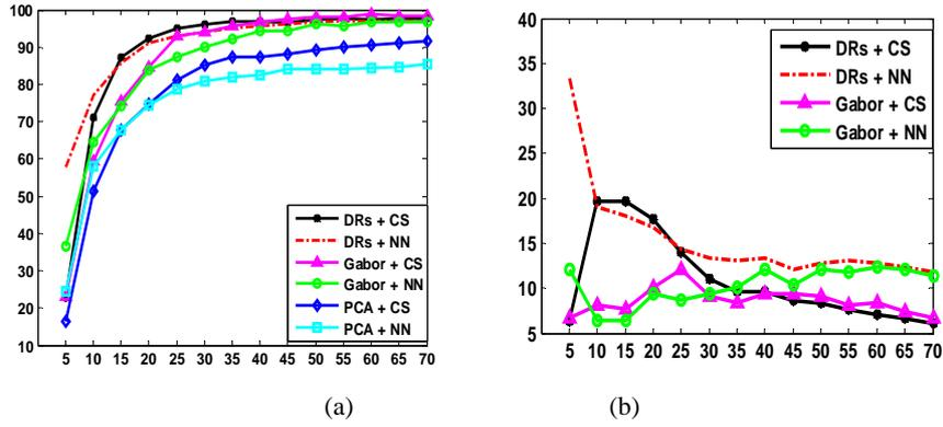
**Fig. 6.** Performance Original palmprint database (a) Recognition performance of different approaches with varying feature dimension (b)Performance comparison between directional representations, Gabor-based and the results obtained by PCA as a reference baseline.
