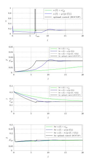
Fig. 3. Time evolution of the suboptimal and approximate optimal processes for  $\gamma_M = \ln(2)/12 \ h^{-1}$  and  $\gamma_R = \ln(2)/24 \ h^{-1}$ . In the top subfigure, the on-off control is not illustrated because of a huge amount of its switchings when the state approaches  $(\hat{p}_{opt}^*, \hat{r}_{opt}^*)$ .
