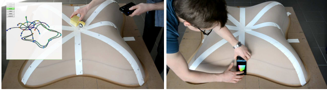
Figure 11: The devices used for data acquisition. Left: the Morphorider (a custom-made device) and a screenshot of the MATLAB acquisition interface. Right: a standard smartphone and the application with a simple acquisition interface.
