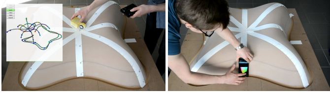
Figure 11: The devices used for data acquisition. Left: the Morphorider and a screenshot of the MATLAB acquisition interface. Right: a standard smartphone and the application with a simple acquisition interface.
