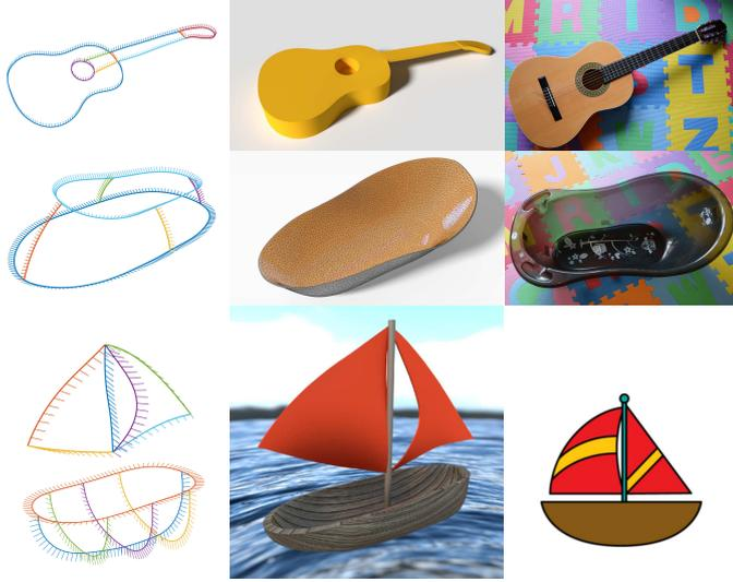
Figure 20: Top: GUITAR and BATHTUB scanned using the Morphorider. Left to right, reconstructed networks, surfaces computed from the networks, the scanned objects. The GUITAR shape was created by extruding the surfaced network. Scanning the translucent BATHTUB was not an issue. Bottom: inspired by the image on the right, we created a 3D model of the SAILBOAT by sketching the network on the left with a smartphone. The lengths were estimated from time of acquisition.
