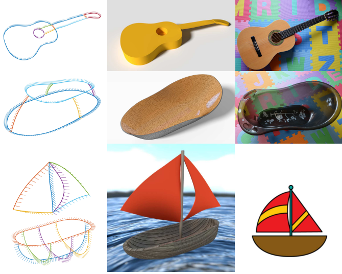
Figure 20: Top: GUITAR and BATHTUB scanned using the Morphorider. Left to right, reconstructed networks, surfaces computed from the networks, the scanned objects. The GUITAR shape was created by extruding the surfaced network. Scanning the translucent BATHTUB was not an issue. Bottom: inspired by the image on the right, we created a 3D model of the SAILBOAT by sketching the network on the left with a smartphone. The lengths were estimated from time of acquisition.
