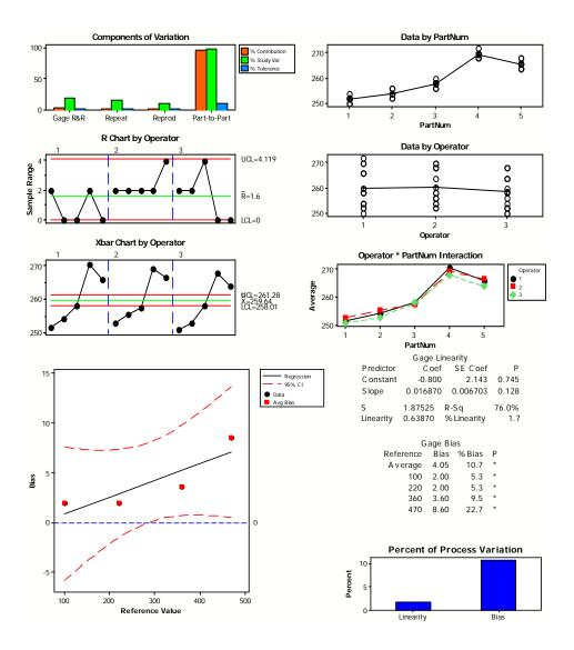
Fig. 1. Details of MSA: gage R&R (up) and linearity and bias study (down)
