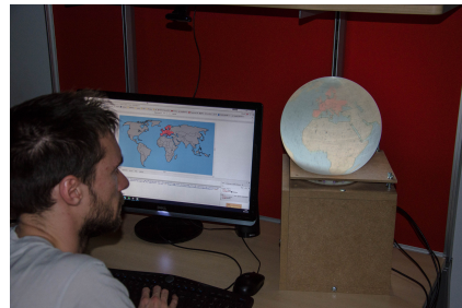
Figure 1. (left) Prototyping a GUI application with a 3D preview on the desktop, and (right) deployment on an interactive spherical display.
