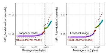
Figure 7. Communication time between two CPUs of the same node of Taurus (i.e., over shared memory). Compared to Figure 1, communications are not only less noisy but can also be almost one order of magnitude faster for large messages. Small messages appear faster over network links than over shared memory because they are sent asynchronously (the duration of MPI\_Send and MPI\_Send does not account for transmission delay).
