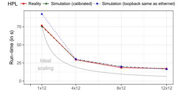
Figure 8. Comparison of simulation results for HPL between a correctly calibrated simulation and simulation that would not account for specific shared memory communication characteristics.
