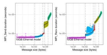
Figure 1. Communication time between two nodes of the Taurus cluster (Ethernet network). The duration of the communication with either MPI\_Send or MPI Recv are modeled as piece-wise linear functions of the message size.
