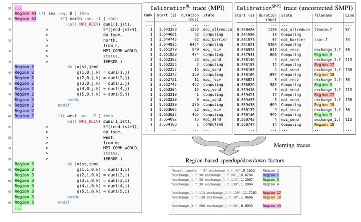
Figure 4. Excerpt of the NAS LU-PB (exchange\_1.f) highlighting code regions between any two MPI cals.
