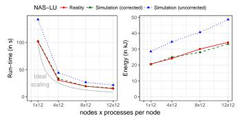
Figure 6. Illustrating the importance of unbiasing the emulation when simulating multi-core CPUs, NAS-LU, class C.
