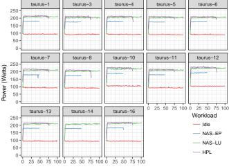
$\begin{array}{c} \text{Time (s)} \\ \text{Figure 3. Power consumption over time when running NAS-EP, NAS-LU,} \\ \text{HPL or idling (with 12 active cores and the frequency set to $2300\,\mathrm{MHz}$).} \end{array}$
