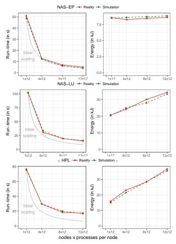
Figure 11. Validating simulation results for NAS-EP, NAS-LU, and HPL, on up to 12 nodes with 12 processes per node.
