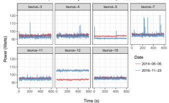
Figure 9. Idle power consumption along time when the frequency is set to 2300 MHz for several nodes of the Taurus cluster in 2014 and in 2016. The Y-axis does not start at 0 to provide a better appreciation of the variations.
