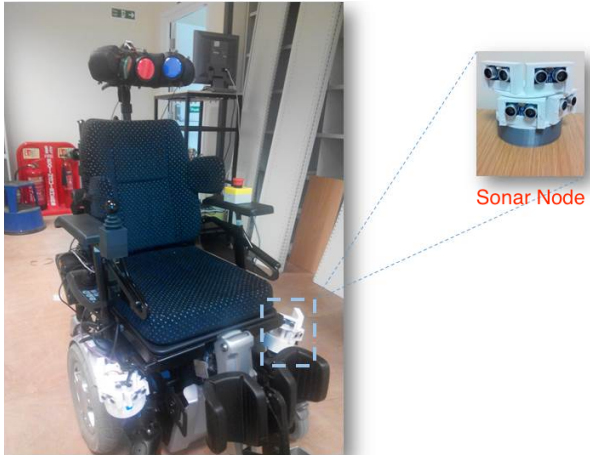
Fig. 1: The smart wheelchair with two sonar sensor nodes at either side of its front. A further two sensor nodes are occluded at the rear of the chair.
