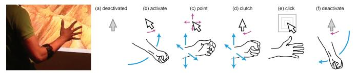
Figure 1: Myo armband (left) and Myopoint interaction (right): (a) initially deactivated; (b) activate by raising clenched fist and releasing; (c) point by moving arm with relaxed hand; (d) clutch with clenched fist; (e) click by spreading all fingers; (f) deactivate by lowering clenched fist and releasing.
