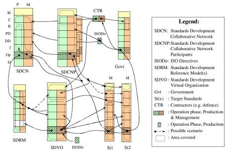
*Life cycle phases:* Id = Identification; C = concept; R = requirements, PD = preliminary design, DD = detailed design, I = implementation, Op = operation, D = decommissioning.*Other aspects:*P = Production / Service, M = management
