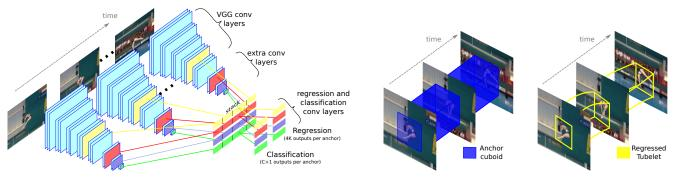
Figure 2. Overview of our ACT-detector. Given a sequence of frames, we extract convolutional features with weights shared between frames. We stack the features from subsequent frames to predict scores and regress coordinates for the anchor cuboids (blue color in the middle). Depending on the size of the anchors, the features come from different convolutional layers (color coded on the left: yellow, red, purple). As output, we obtain tubelets (yellow color on the right).
