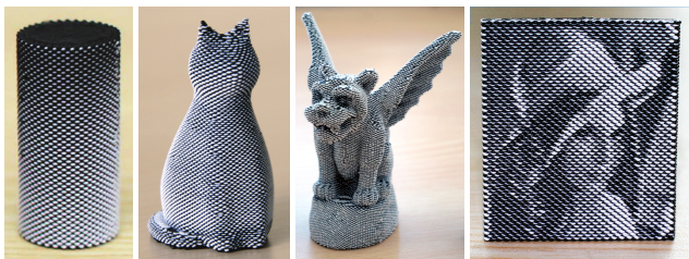
Figure 16: Producing continuous tone imagery by color mixing on multi-filament printers. Image courtesy of [RCM*14].
