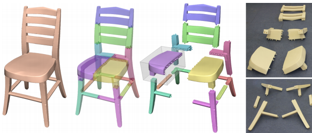
Figure 18: A 3D object is partitioned into reassemblable parts that can be printed. Image courtesy of [LBRM12].
