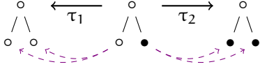
Fig. 2. Using obits to deduce origins. We represent the obits with colours: \circ are nodes of obit 0, \bullet are nodes of obit 1. We apply two transformations \tau_1 and \tau_2 on an input tree (here in the middle): \tau_1 replaces its right leaf by a copy of the left one, while \tau_2 replaces its left leaf by a copy of the right one. Visually, “turning on” an obit in the input makes it possible to visualise all output nodes that depend upon it.
