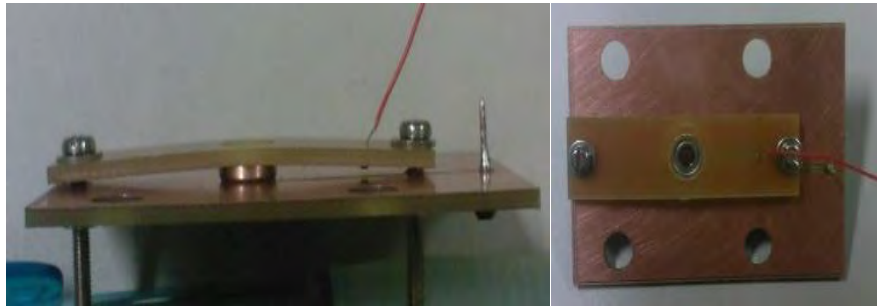
Fig. 18. Board uses to mount and test the liquid lens
