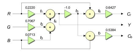
Fig. 3. ITU RGB to YCrCb converter.
