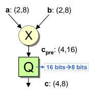
Fig. 2. Quantization of a multiplier.
