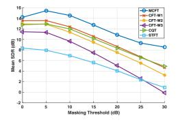
**Fig. 2.** Mean SDR for 2D and 4D representations versus masking threshold. 3 out of 9 patch sizes used in CFT computation are shown:  $W_1$  (2 × 128) (best),  $W_2$  (4 × 64) (default), and  $W_3$  (8 × 32) (worst).
